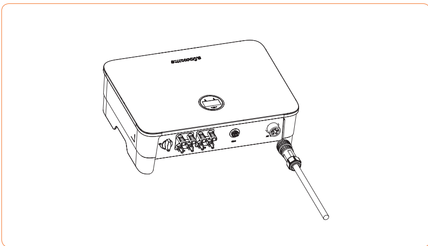
Figure 4-24 Connect the AC connector
